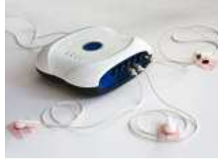
Figure 1: multifrequency (1 to 1000 kHz) impedancemeter Z-Métrix ® .
